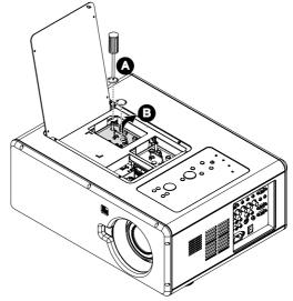
**3.** Pull firmly on the module handle in the direction shown to remove the lamp.
